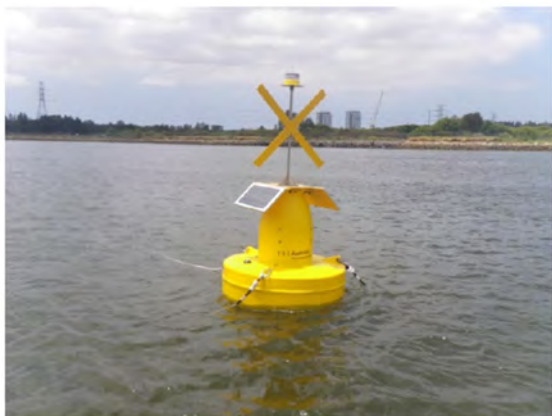
Figure 3: Buoy to be used for housing monitoring stations in open water.
